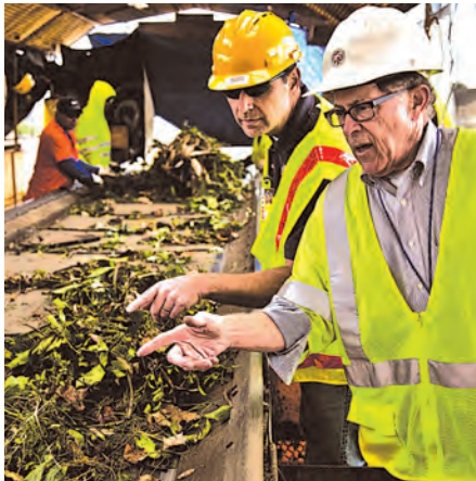
From April 2010: Paul Blount, Operations Manager (right), describes to Club CEO John Hawkins, how solid contaminants (bottles, paper, etc.) are picked by hand from the raw mulch, along a conveyor belt.
