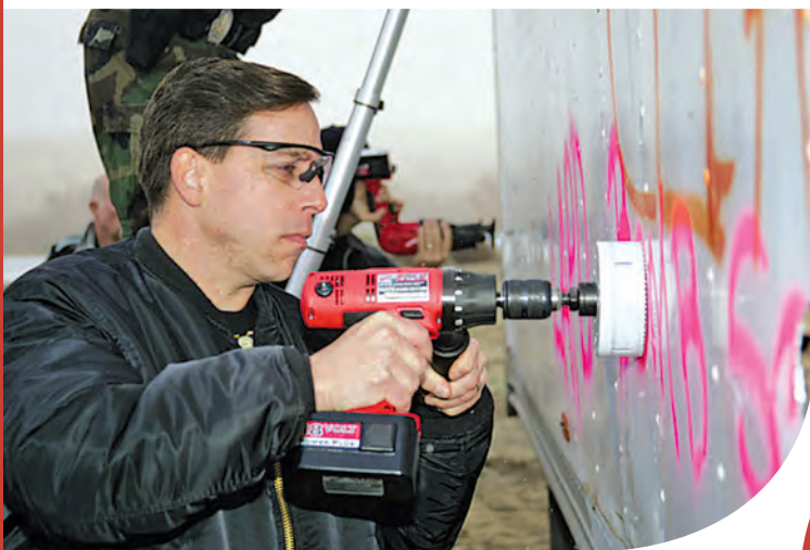
Sgt. Michael Salinaz, the Officer in Charge of the Bomb Squad, cuts through a panel truck's wall so the squad can insert a camera and examine the truck's contents.
