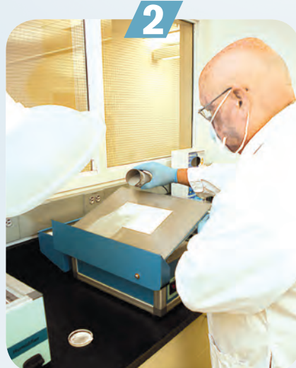
A thin plastic Mylar sheet is placed on top of the sheet of paper to protect the evidence. The sheet is made smooth with a roller. With the machine on, air pulls the sheet to the bed, and a slight electrostatic charge is given to the sheet. Then, a special toner is poured on top of the blank sheet (covered in plastic).
