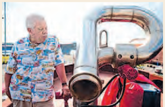
Frank Borden examines one of the stainless steel pipes that fed one of the boat's water cannons.
