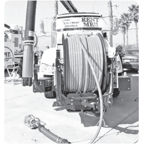
Combination machines (trucks), which clean and vacuum out waste systems.
