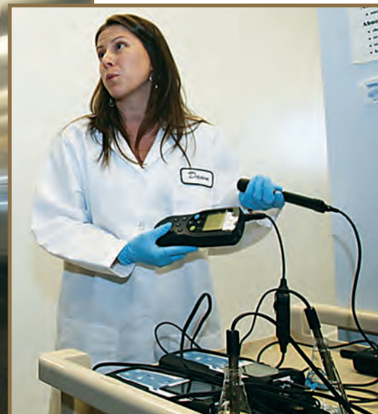
Water quality measurements (e.g. salinity, pH, dissolved oxygen) are performed using probes throughout the duration of the toxicity tests.
