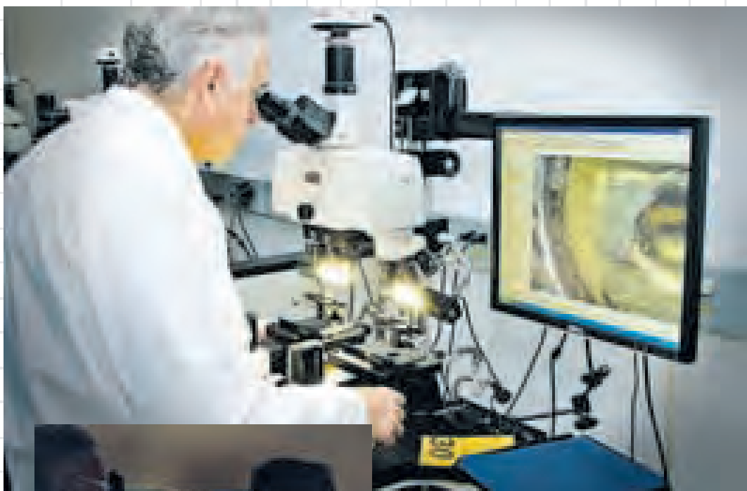
Daniel Rubin, Criminalist, is comparing two fired cartridge cases to determine whether or not they came from the same source. He identifies these as matching, as coming from the same weapon.
