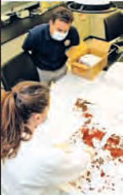
Jessica Bullock, Criminalist, 1 year of City service, examines a shirt in an ongoing case for bullet entry and exit holes. She has placed a marker with the letter "A" where she has determined the bullet punctured the shirt. With her is Club CEO John Hawkins.
