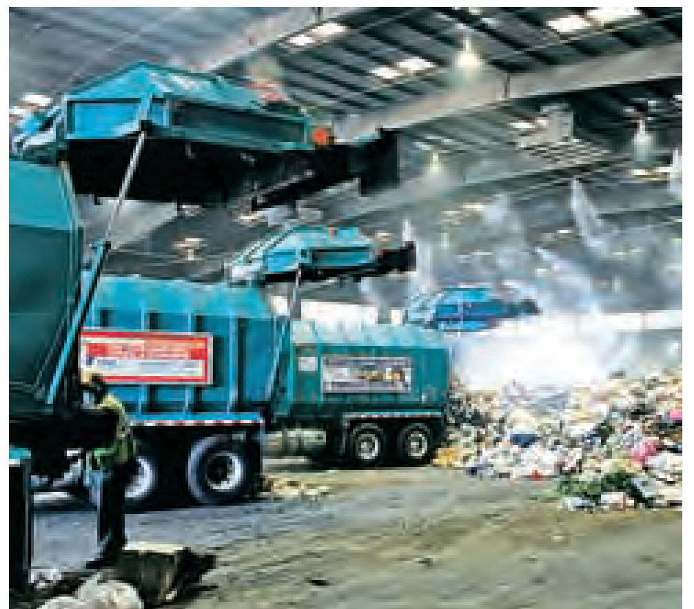
Three curbside refuse collection trucks line up on the floor of the transfer station and dump their contents.
