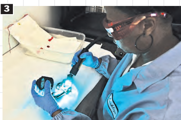
3 After the chemical wash, the weapon is viewed with special lighting to locate any latent print evidence.
