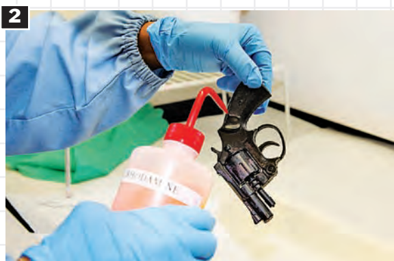
2 Special chemicals are applied to the weapon to develop possible latent print impression evidence that was left behind.
