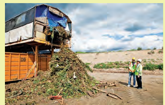
b) The coarse material is then piled at the end of the picking station. At this point, it's called raw mulch.
