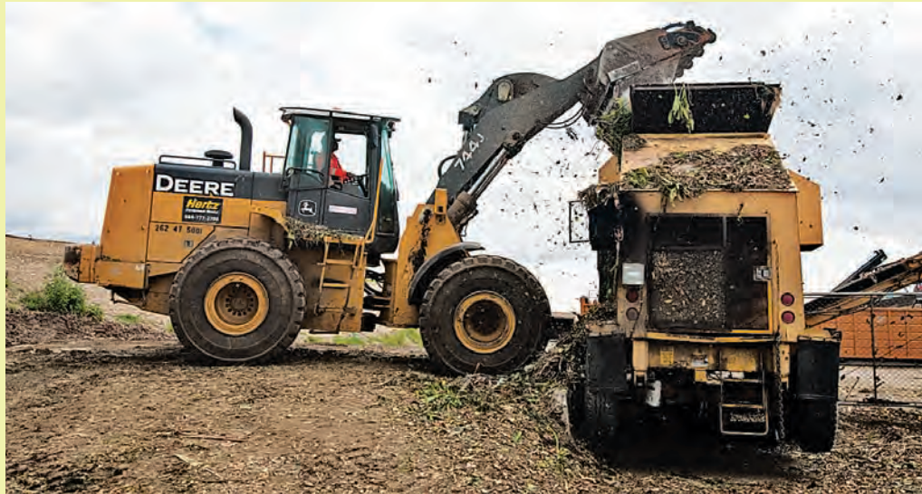
Anceo Francisco, Equipment Operator, dumps raw mulch into the trommel screen machine.
