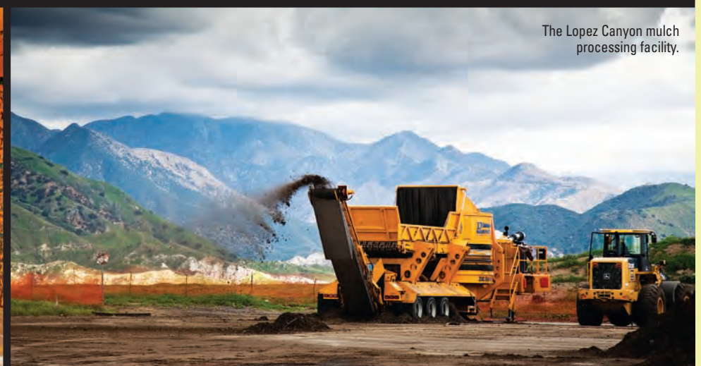
A chute collects the solid contaminants – bottles, paper, etc. – from the yard trimmings before the grinding begins.
