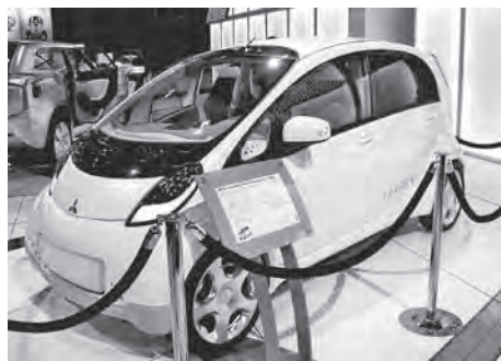
Mitsubishi i-MiEV or Mitsubishi innovative Electric Vehicle uses a 16-kilowatt-hour lithium-ion battery. The four-seat, five-door hatchback is one of the first of a wave of highway-capable electric vehicles. This new model gets 60-100 miles on a full battery.
